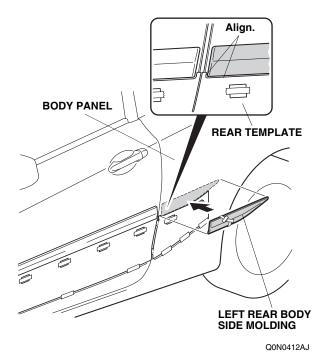
15. Press on the left rear body side molding firmly with the palm of your hand while removing about 50 to 100 mm (2.0 to 3.9 in.) of the adhesive backing at a time.
