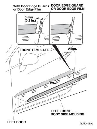
11. Press on the left front body side molding firmly with the palm of your hand while removing about 50 to 100 mm (2.0 to 3.9 in.) of the adhesive backing at a time.
