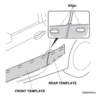
8. Using two alcohol wipes, clean the surface of the left door and body panel above the templates where the body side moldings will attach. Allow the alcohol to dry before installing the side moldings.
