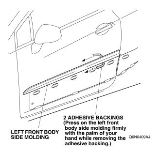
12. Using a rubber roller, apply firm pressure while rolling to set the adhesive. Apply firm pressure especially at the ends.
