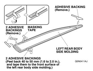
14. Align the edges of the left rear body side molding with the edges of the rear template, and attach the left rear body side molding to the body panel.
