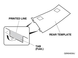
5. Align the two tabs on the rear template against the front edge of the body panel.
